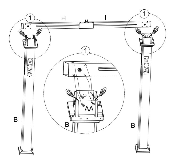
1. Place assembled short crossbar set (H, I) over the post (B), insert screw 1 (AA) through post (B) secure with short crossbar set as figure shown.
