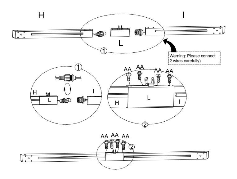
1. Insert short crossbar A (H) into center connector (L), then connect (H) and (I) wires in clockwise as figure 1 shown, insert screw 1 (AA) through center connector (L) to secure short crossbar A (H) and short crossbar B (I) as figure 2 shown.
