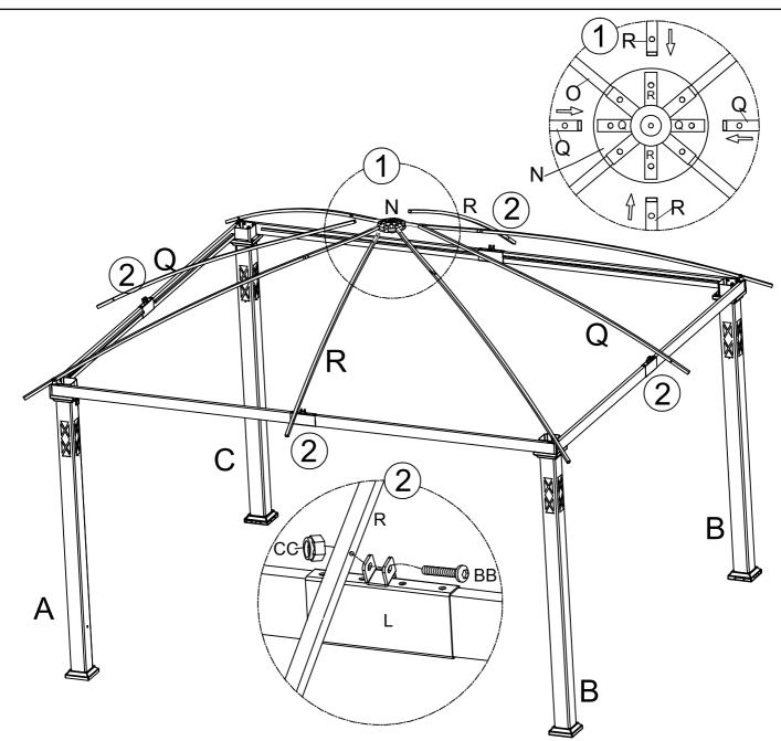
Insert short roof tube (R) into roof connector (N), then secure the end section of short roof tube (R) with center connector (L) by using screw 2 (BB) and bolt nut (CC) as figure 2 shown.
