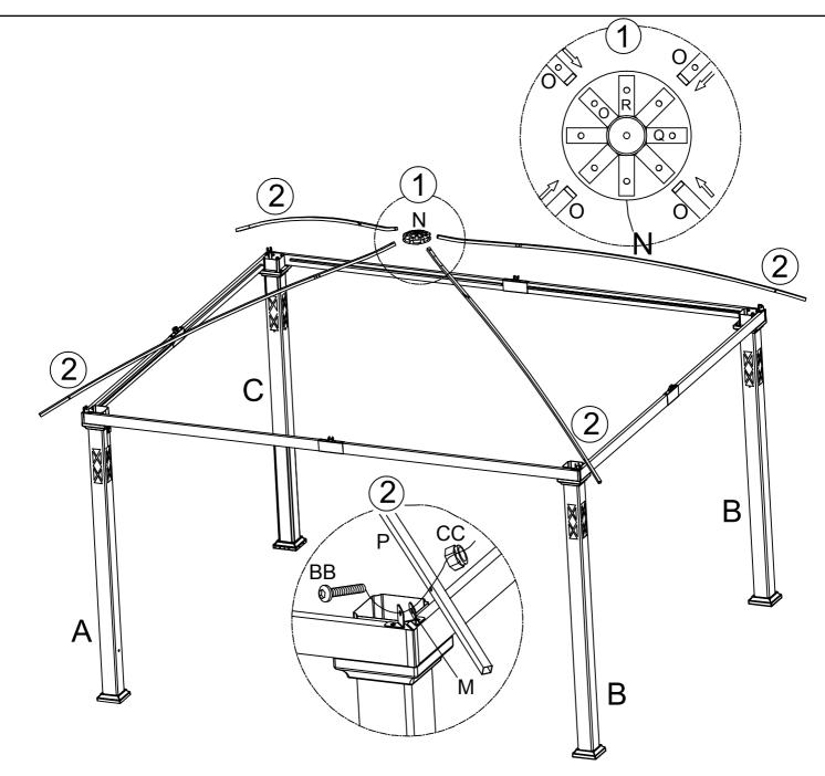
1. Insert corner short roof tube (O) into roof connector (N) as figure 1 shown, then secure corner roof tube (P) with corner connector (M) by using screw 2 (BB) and bolt nut (CC) as figure 2 shown. Repeat for all remaining roof tube sets (O & P).
