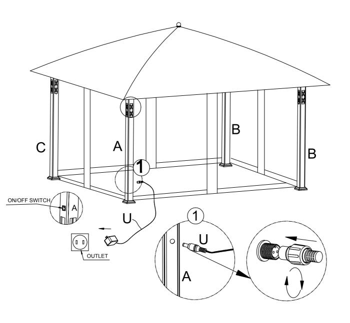
1. Please ensure all of the wires are connected properly then connect AC adapter (U) on the bottom of post (A) in clockwise.
