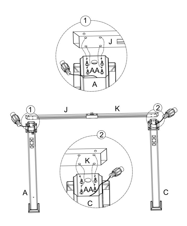
1. Place assembled short crossbar set (J, K) over the post (A) and post (C), insert screw 1 (AA) through post (A) secure with short crossbar (J) as figure 1 shown.
