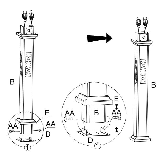
1. Insert base cap (E) into post (B), then using screw (AA) secure base flange (D) on the bottom of post (B).
