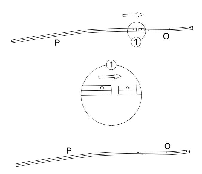
1. Insert corner short roof tube into corner roof tube (P) as figure shown. Repeat for remaining corner short roof tube (O) and corner roof tube (P).
