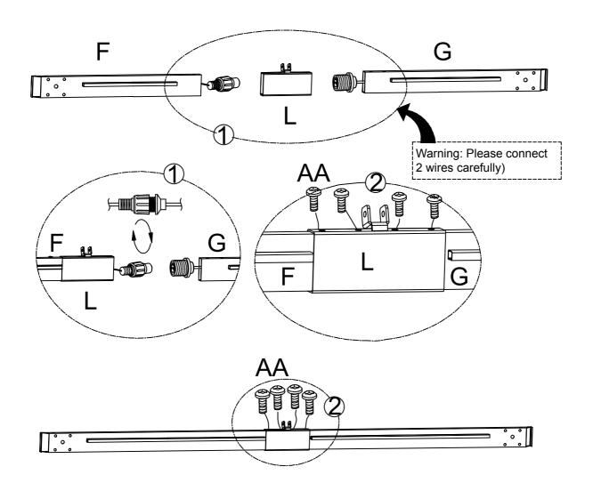
1. Insert long crossbar A (F) into center connector (L), then connect (F) and (G) wires in clockwise as figure 1 shown, insert screw 1 (AA) through center connector (L) to secure long crossbar A (F) and long crossbar B (G) as figure 2 shown.
