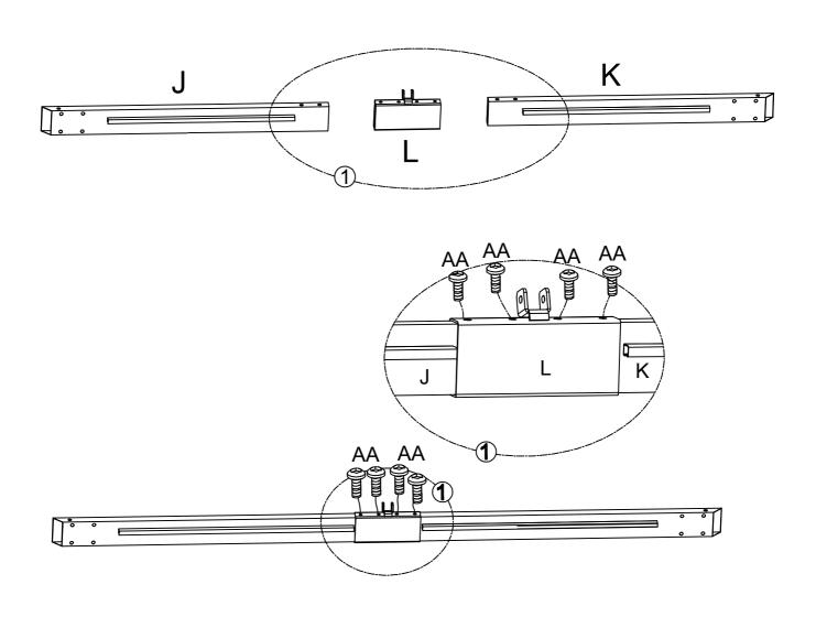
1. Insert short crossbar C (J) and short crossbar D (K) into center connector (L), then insert screw 1 (AA) through center connector (L) to secure short crossbar C (J) and short crossbar D (K) as figure shown.
