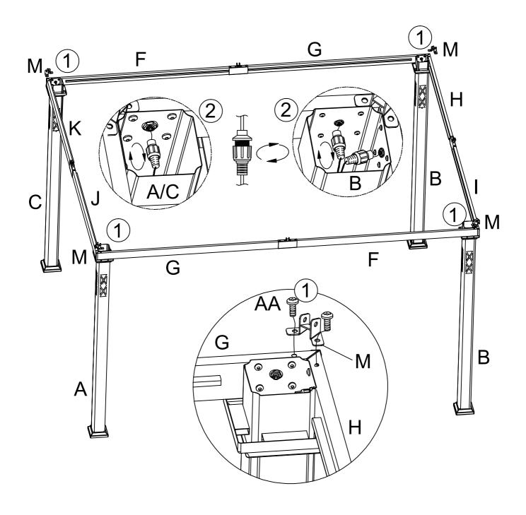
1. Secure corner connector (M) onto crossbar (G) and crossbar (H) by using screw 1 (AA) as figure 1 shown.
